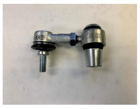
**Step E**Insert M10 washer and locking nut
